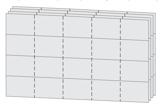
Rotate 90 degrees and cut up to 5 sheets (stacked) vertically at 12" (on center)
